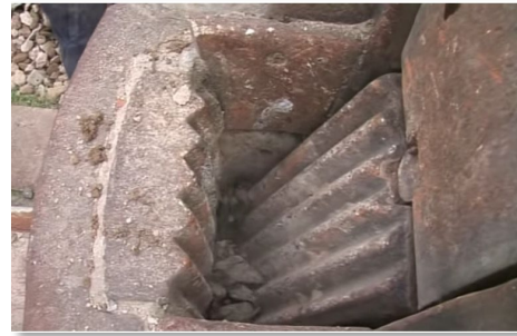
Rock hopper and jaws crushing stone [2011 demo of Blake Stone Breaker - https://youtu.be/ho5vcrAkhwg ]
